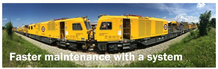
Fig. 1: RORUNNER system for the London Elizabeth Line consists of two train formations, each with two track vehicles and one transport transport wagon.
