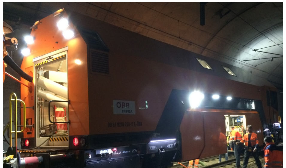
Fig. 7 The two-floor ROMIS Compact is particularly suitable for use in constricted spaces.
