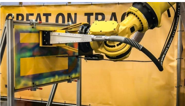
Fig. 3. The most environmentally friendly way of removing graffiti: the dry ice pellets sublime completely after use.
