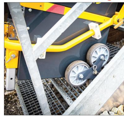
Robel rail/road trolley has been specially designed for easy transport of the high capacity battery pack and other materials, which might be required at the worksite.
