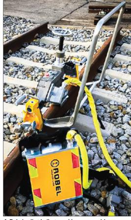
A Robel rail grinding machine powered by a 2kWh battery.
