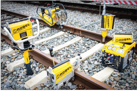
welding joint grinding machine and a hybrid railhead profile grinding machine - that can either be driven by a 2kWh battery, a 6kWh battery or a power supply.
