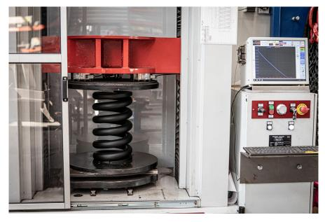
Fig. 4: A calibrated measurement rig tests the primary and secondary suspension of the bogies.
