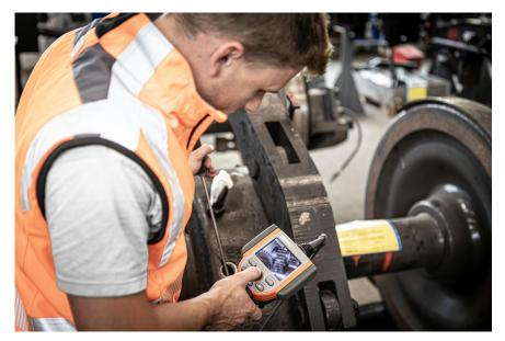
Fig. 2: Endoscopy of the wheelset shows the condition of the distribution gearboxes in detail
