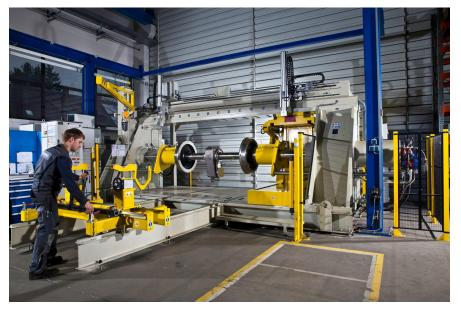
**Fig. 6:** Pacemaker and precision instrument: The wheelset press ensures and records quality and function of the critical connection between wheels, brake disks and shafts.
