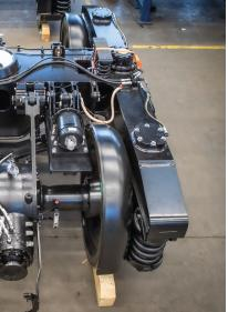
Fig. 1: Bogie of a 09-3X tamping machine before and after overhaul Source of all Figures: Robel
