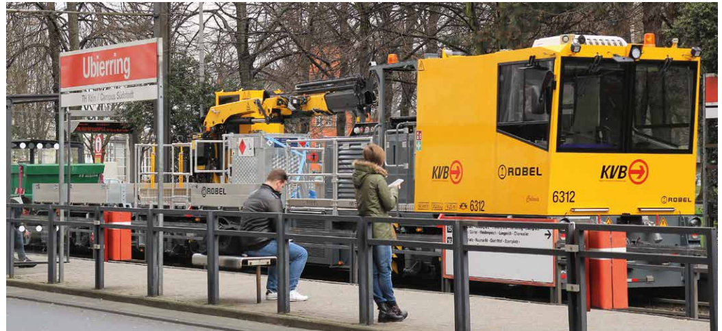
Fig. 8: The transport system for Kölner Verkehrsbetriebe is used on the underground as well as on public roads.
