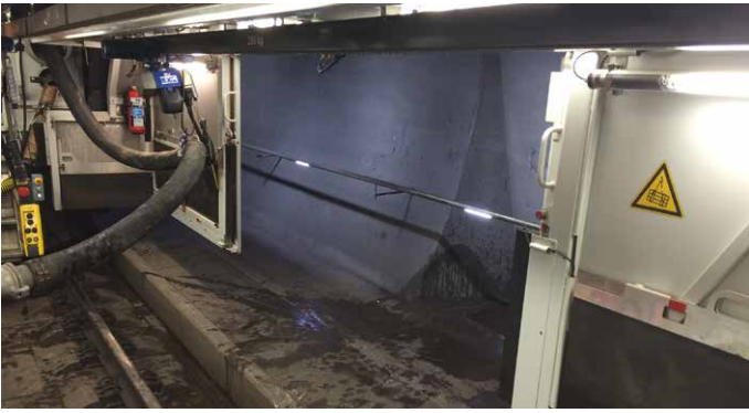
Fig. 3: The open side wall of the Mobile Maintenance System facilitates the protected access for cleaning of drainage channels in tunnels.
