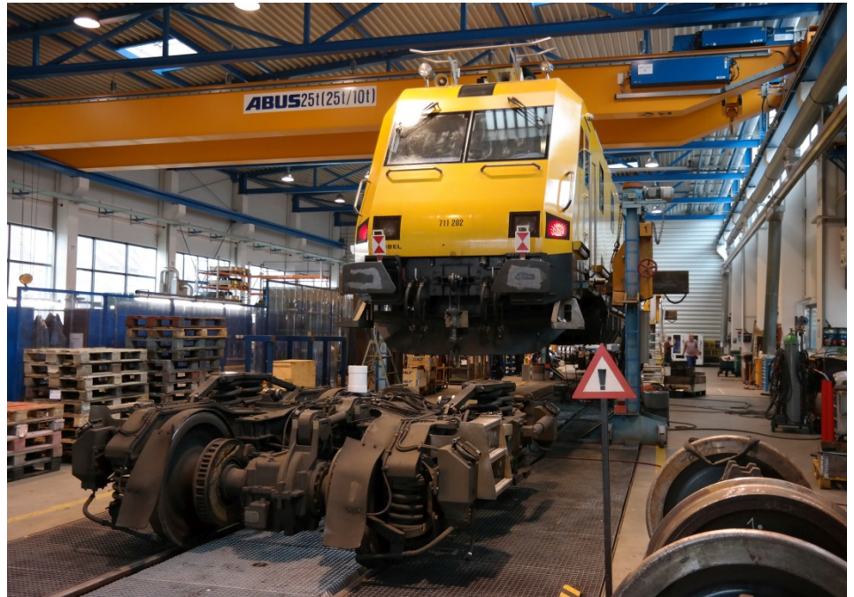
Fig. 6: Dismantling the old bogie during an overhaul
