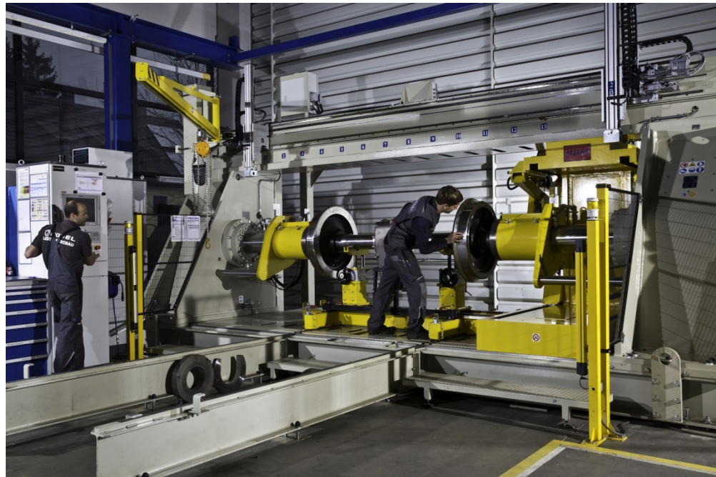
Fig. 2: Axle press for automatic press-fitting and pressing off wheels with digital monitoring and recording
