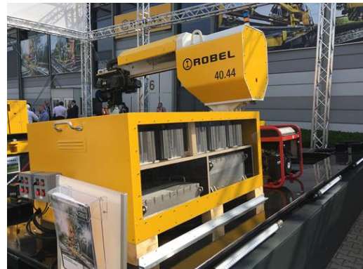
Fig. 4: The Hybrid Power Pack optimises generator output and so reduces fuel consumption and emissions.
