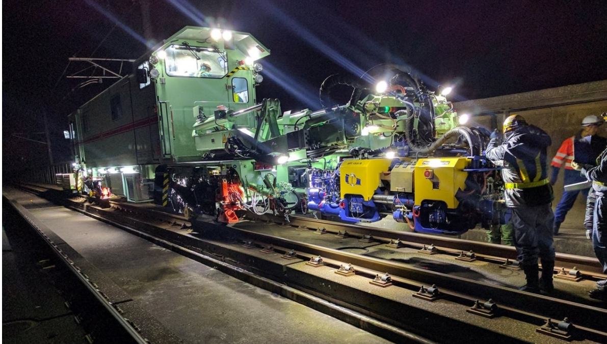
Fig. 11: The mobile APT welding robot from Plasser & Theurer is part of the REX-S 1200 Rail Exchange System used on the Shinkansen.
