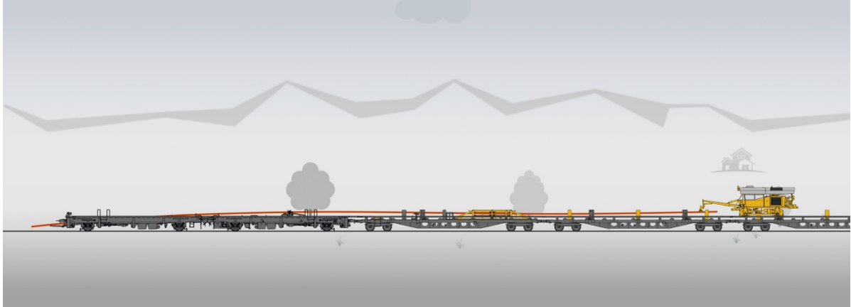
Fig. 8: REX-S, consisting of chute wagon, transport unit and rail manipulator, can unload a pair of 180 m rails in two minutes and load it in four minutes.
