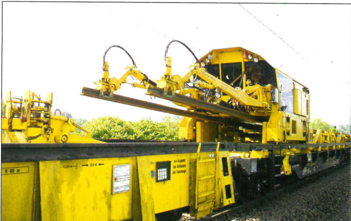
The train's manipulator unloading rail (above) and inside its cabin (right).
