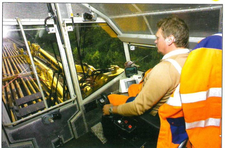
The train's manipulator unloading rail (above) and inside its cabin (right).
